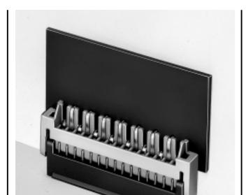
Hinge type board to board connectors which allow mated PCB's to move 90° in respect to one another while electricity is turned on. The hinge compensates for slight misalignments between circuit boards to assure a secure connection even if the boards are laterally out of line.
